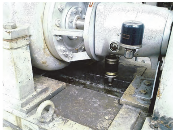
BOS Drain Bottle/BS&W Bowl on Centrifugal Pump running on Royal Purple Synthetic Oil
