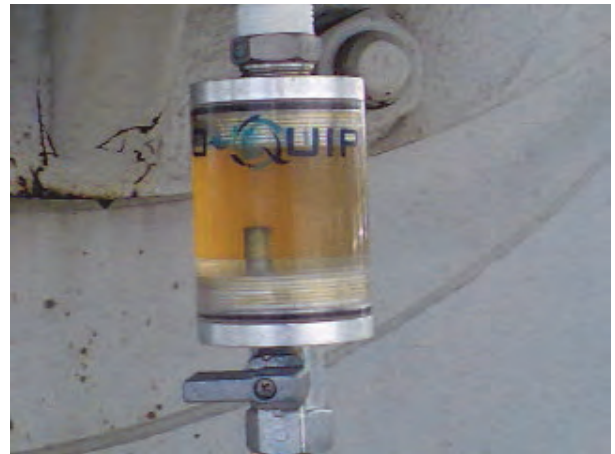
BOS Drain Bottle/BS&W Bowl showing Oil and Water Separation
